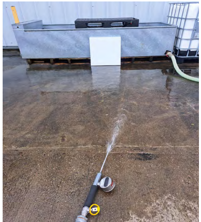
EFW Panel During Water Ingress Testing
