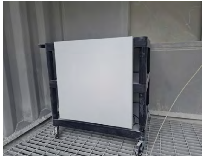
EFW Panel During Dust Ingress Testing
